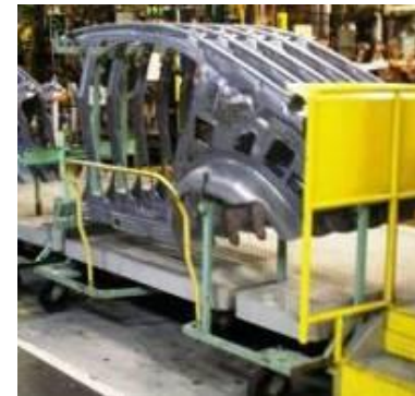
Racks on Wheels
